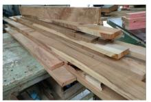
Description:English elm timber.Common uses are furniture, doors, and kitchens. Historically used for making chariot<br/>wheels, due to strong cross grain dimension strength.Dimensions<br/>and price:150mm x 25mm = \$21.00 per metre<br/>150mm x 55mm = \$36.00 per metreSAWN200mm x 25mm = \$34.00 per metre<br/>220mm x 25mm = \$36.00 per metre<br/>220mm x 35mm = \$36.00 per metre
