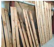
**Description:** Highly decorative, honey coloured timber. Finished with an interlocking tongue and groove. Uses include decorative wall and ceiling lining and can also be used for soffit linings in sheltered areas (moderately durable).
