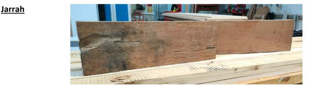
**Description:** An Australian hardwood that is both incredible heavy and dense. Suitable for in ground and above ground uses. Has a rich red/ brown colour, especially when polished.
