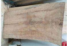
**Description:** A heavy and dense NZ hardwood that is often used for flooring. Also used for built-in furniture, internal joinery and panelling. It is a very stable in nature which is great for ensuring its finished product stays true to the original design
